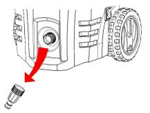
Clean the nozzle with the needle clean-out tool provided. Remove the spray lance from the gun. Remove any dirt from the nozzle hole and rinse.
