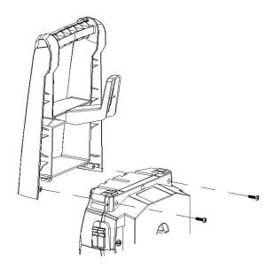
2) Installing the Spray wand holder with two screws.
