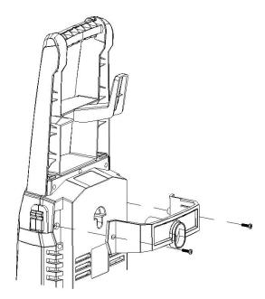
3) Slide the trigger gun holder on the side of the machine.
