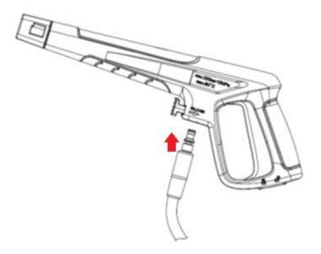
To remove the hose, switch off and unplug the appliance. Push the release button and pull out the hose.
